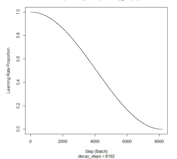
Essentially the cosine function for inputs in [0, pi] shifted to the output range [0, 1]; can be combined with "restarts"
